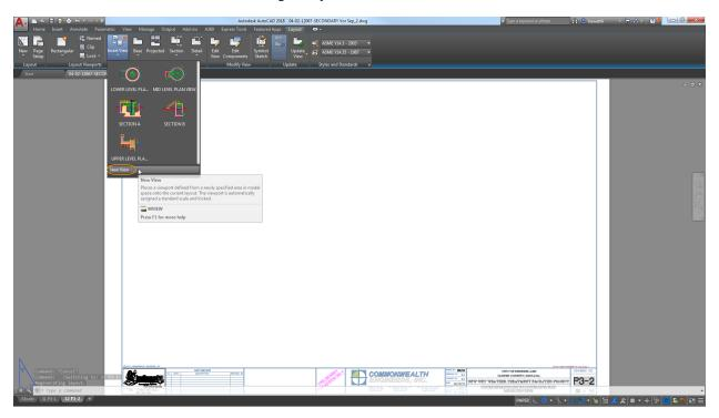
This allows you to specify the view area in model space and then immediately place the view on the layout. If the drawing contains no named views, selecting the Insert View tool from the Layout ribbon tab automatically launches the New View behavior.
