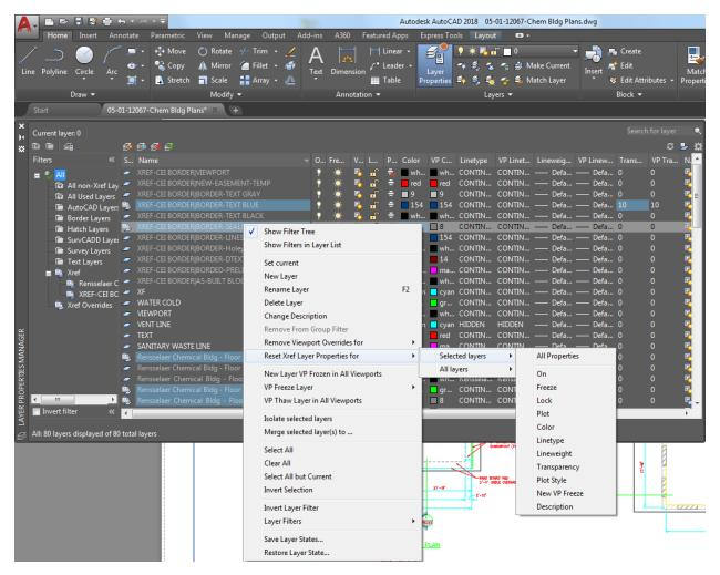
Additionally, a new XREF option in the -LAYER command offers command line access to remove Xref overrides, and a previously hidden option in the VPLAYER command for removing Viewport Overrides [reMoveoverrides] has been exposed.
