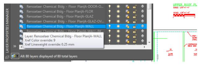
A new toggle in the Layer Properties Manager makes it even easier to identify Xref layer overrides by applying a background color to any and all layers and properties with overrides—including both Xref and viewport overrides.
