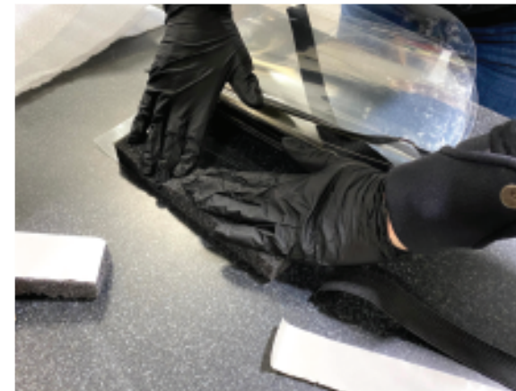
Center foam along top edge of shield and press down to get the adhesive to stick.
