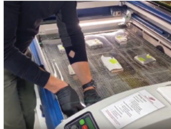
Weigh down each shield to avoid curling. Experiment with speed and power of laser.
