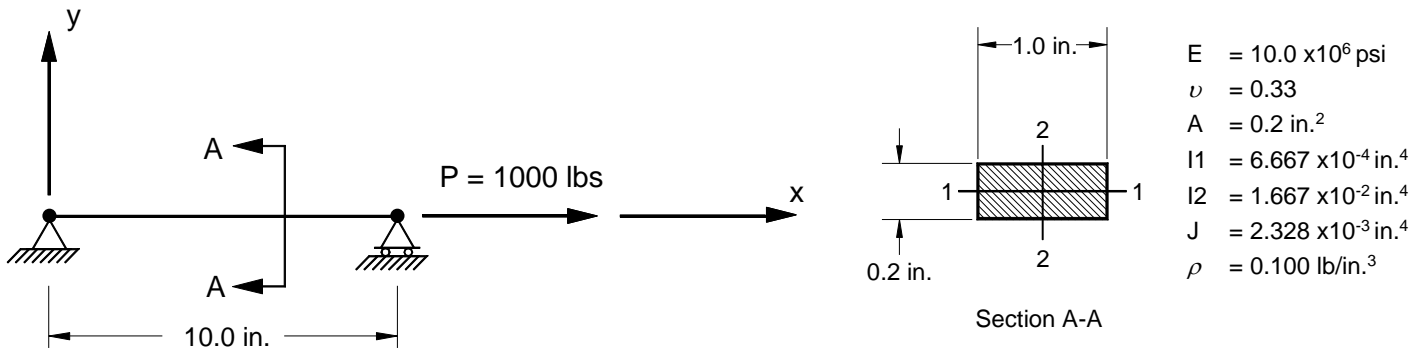
Figure 11-1. 2-D Simply-Supported Beam Example Problem.
