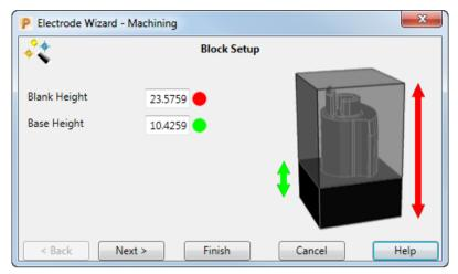
**Blank height** — The height of the electrode machining material.
