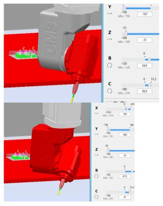
When a collision occurs, the colliding parts of machine are coloured and a warning message is displayed:
