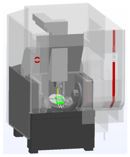
Now you can create the <machine\_part> definitions. There are two <machine\_part> definitions: one for the head of the machine and one for the table. This example defines a machine tool with a Table-Table configuration.
