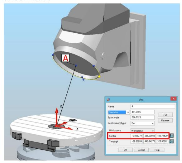
Double clicking on arc. The point  $\bf A$  is centre of rotation with coordinates:  $X=-0.098279\ Y=285.29986\ Z=483.74620.$
