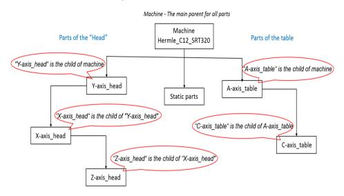
This example begins with the Y axis. The component model that makes up the Y axis acts as the parent component upon which the remaining axial components for X and Z are attached. You must give each axial component a definition:
