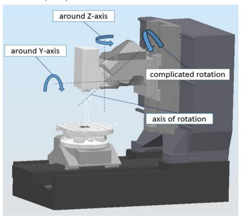
Such rotation is complicated because it consists of two rotational movements (around Z-axis and around Y-axis).
