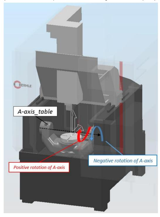
Let us open A-axis\_table and C-axis\_table in PowerShape. Then you can create new Local Coordinate System (LCS number 1) at x=0 y=0 z=0. This coordinate system duplicates the Global Coordinate System (GCS). See below.
