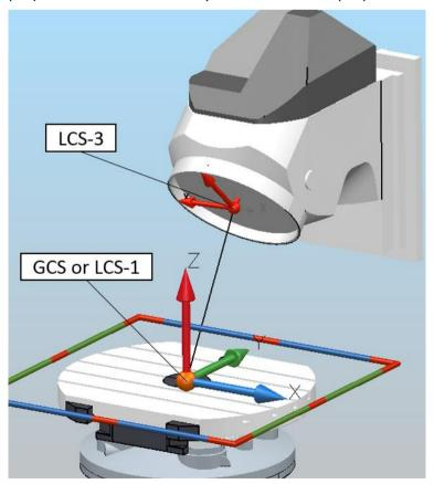
By using activated LCS-3 create short line (start point x=0; y=0; z=0; and end point x=0; y=0; z=1)
