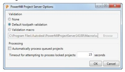
The validation options enable you to set the criteria used to assess whether a project is considered safe to be machined and, therefore, if the project is processed successfully or not.
