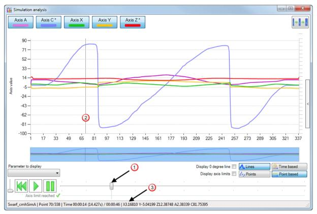
Moving the slider to position 1 displays the location on the graph 2 and details of the location are displayed at the bottom of the window 3.
