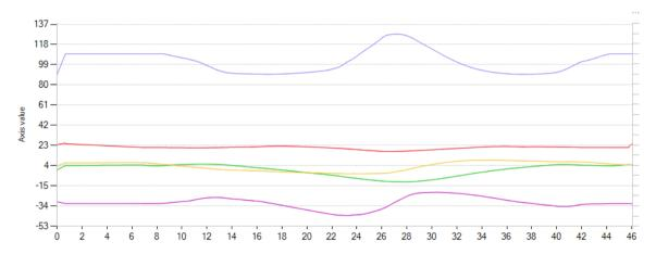
**Graph** — Displays a line graph of each machine tool (or robot) axis. Each axis is drawn in a different colour. Move the cursor over the line graph to display its point information.
