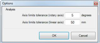
Axis limits tolerance (rotary axis) — Enter the angular tolerance to detect an axis limit. For example, if the machine tool has a maximum angular limit of  $\pm 90^{\circ}$  and you enter a value of 5 here, the simulation analysis shows an axis limit is reached at  $\pm 85^{\circ}$ .
