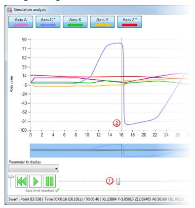
As you move the slider, the simulation is updated in the main PowerMill window. This shows an almost  $180^{\circ}$  swing of the C axis over a small distance on the part.
