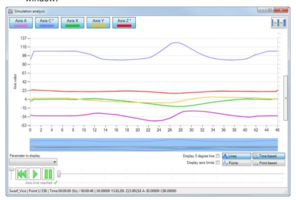
This produces better control of the C axis. Although the C axis rotates around 24 to 32 seconds, this is acceptable because it is controlled rotation around the part.
