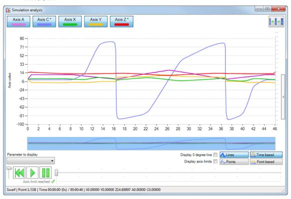
You can see a line graph for each individual axis. Each axis is drawn in a different colour. In this case most of the axes are well-behaved, except for the C axis which is the rotary table.
