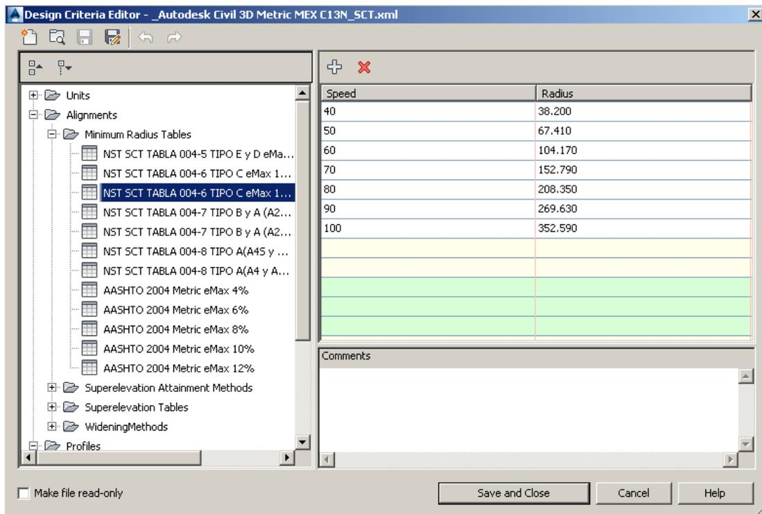
The screenshot shows the 'Design Criteria Editor' window for 'Autodesk Civil 3D Metric MEX C13N\_SCT.xml'. The left pane shows a tree view with 'Minimum Radius Tables' selected. The right pane displays a table with 'Speed' and 'Radius' columns. The table contains data for speeds from 40 to 100 km/h. Below the table is a 'Comments' field and buttons for 'Save and Close', 'Cancel', and 'Help'.
